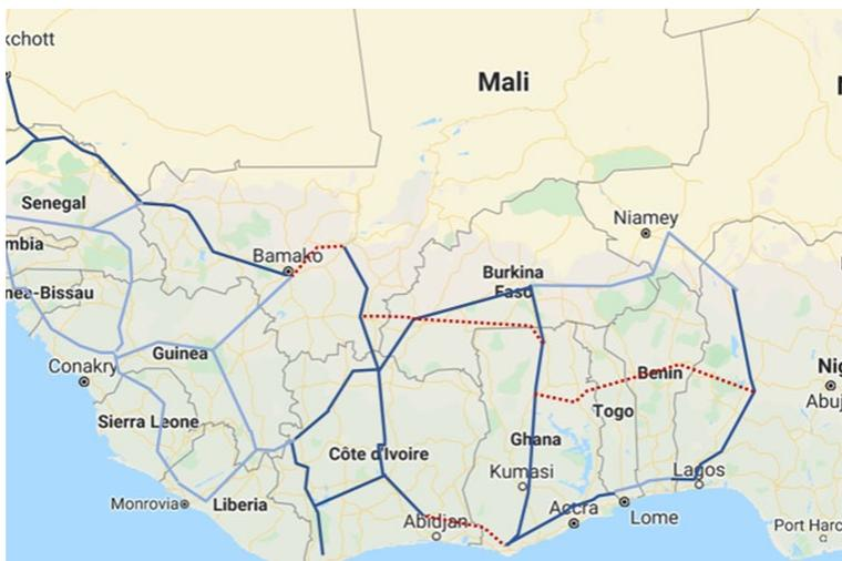
*Note: dark blue lines represent current transmission lines; light blue lines represent those that are close to being made operational, under construction, or for which funding is secured; dotted lines represent future expected transmission lines. Source: The World Bank*
